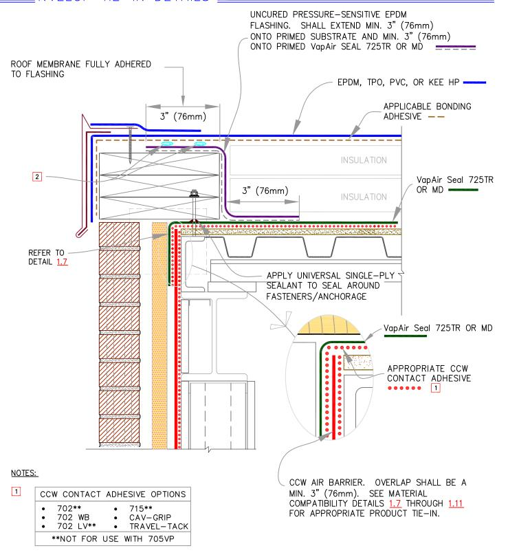
\*\*NEEDED ONLY WHEN ROOF MEMBRANE IS PVC OR KEE HP\*\* APPLY TWO CONTINUOUS BEADS OF UNIVERSAL SINGLE-PLY SEALANT SANDWICHED BETWEEN UNCURED EPDM FLASHING AND PVC/KEE HP.
